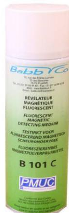
**B 101C**, generator of 400 mL aerosol. Expanded granulation of powder: 0,5 à 10 µm for a good developer’s versatility: efficient detection of sharper defects as wider ones. Granulation pick to 4 µm for a reduced noise even on rough working surfaces. **NON-FLAMMABLE** multi positions **AEROSOLS**.
